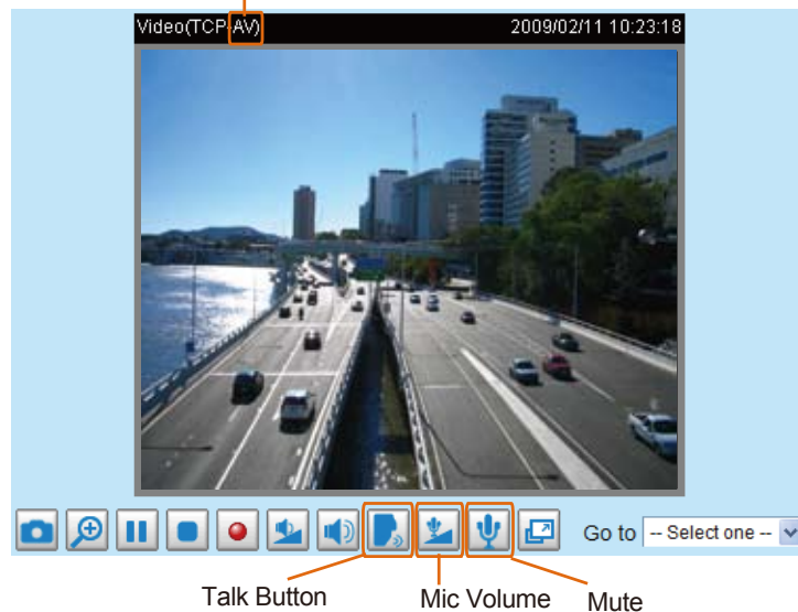
Audio is being transmitted to the Network Camera
